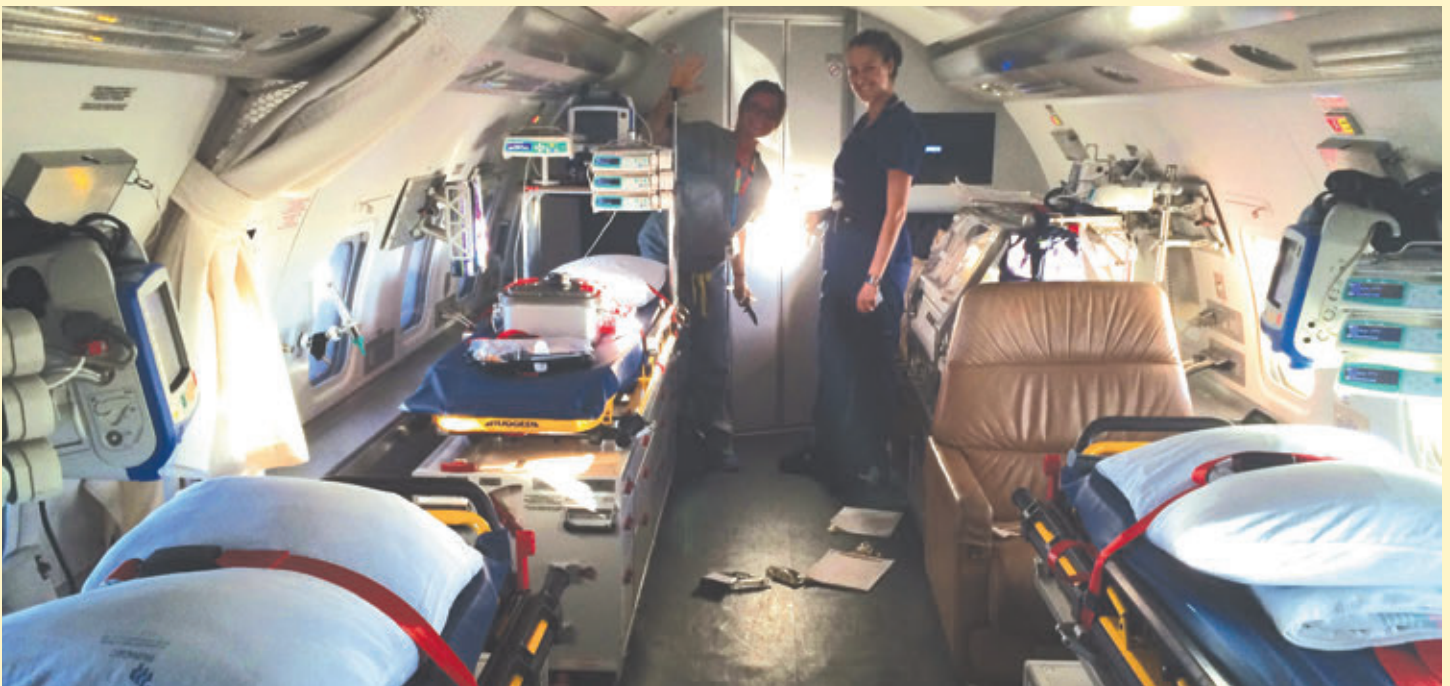
“The Challenger jet was fully equipped like a mini-hospital,” says Dr. Malenfant-Rancourt. The jet has specialized medical equipment, including three stretchers and an incubator, and can provide care for several patients at the same time.
